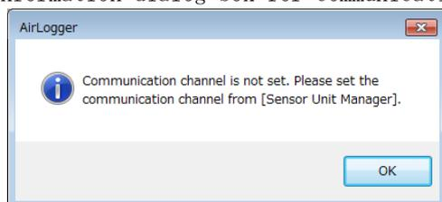
The communication frequency channel of the PC-side communication unit is configured to the default setting. It should be configured to the appropriate setting. Click the [OK] button, and the Sensor Unit Management window (see Section [6.1 Sensor Unit Management window](#)) appears. Set the channel in accordance with Section [6.5 Setting the communication frequency](#).
