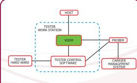
Advantest's patented single wire test cell solution.
