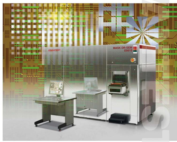
The E5610 is a MASK DR-SEM<sup>1)</sup> for reviewing and classifying ultra-small defects in photomask and blanks.
