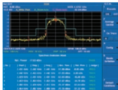
Example of S.E.M. measurement for wireless LAN
