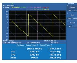
Overlay display: Phase vs. time comparison of two signals
