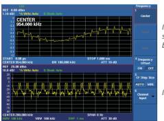
Inverter noise superimposed on broadcast waves
