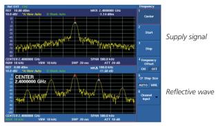
Example 6: Measurement of a 2.4-GHz high-frequency power source signal and reflective wave
