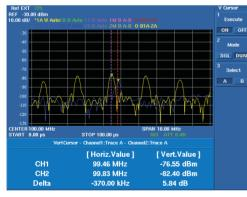
Overlay display: FFT comparison of two signals
