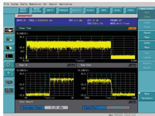
Power Time & Ramp Measurement画面
