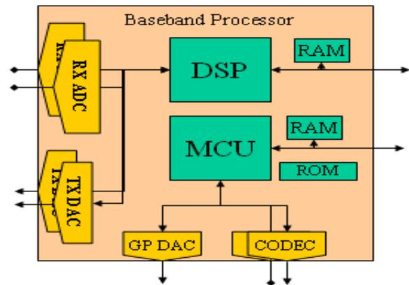
**Figure 1: Baseband Processor Block Diagram**
