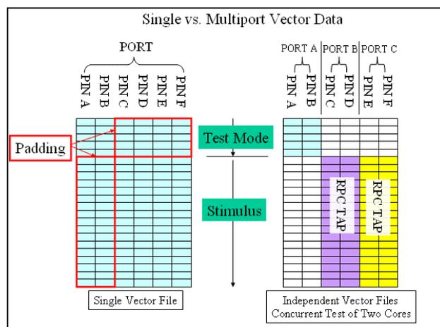
**Figure 5: Multiport-Based Test Vector Segmentation**
