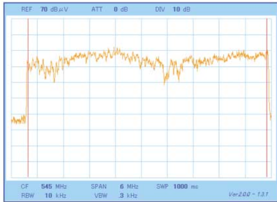
図3 振幅周波数特性測定結果 Fig.3 Results of Modulated Frequency Response Measurements
