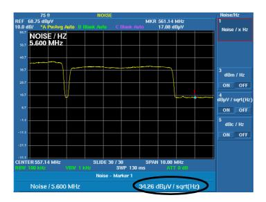
Figure 4-22 Measurement Display for Noise Power Converted into 5.6 MHz
