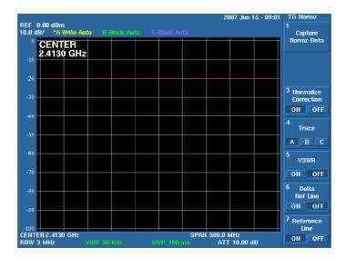
3. Connect the DUT to the TEST port of the SWR bridge. Press *VSWR ON/OFF(ON)*.
