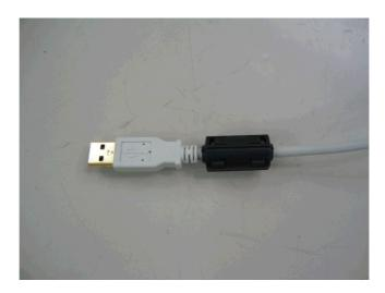
Figure 3-3 Attachment of a Ferrite Core 1
