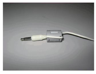
Figure 3-4 Attachment of a Ferrite Core 2
