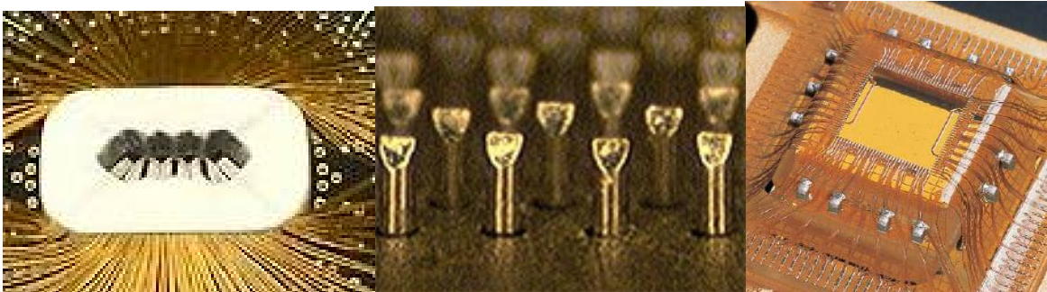
Figure 3. From left to right: Cantilever, Vertical and Membrane Probe (courtesy of Cascade Microtech Inc.).
