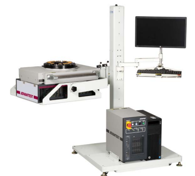
P-Model set up with Manipulator (provided by 3 rd party supplier)
