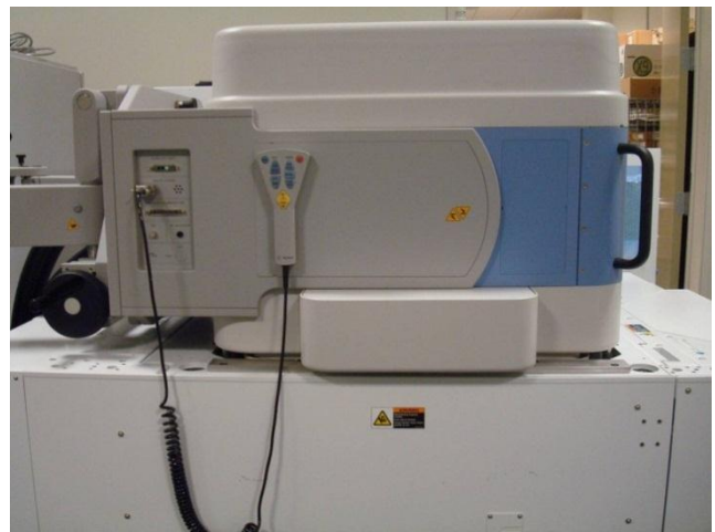
Figure 1. Verigy V93000 SOC Tester Docked to a Prober in the V93000 Direct Probe Configuration
