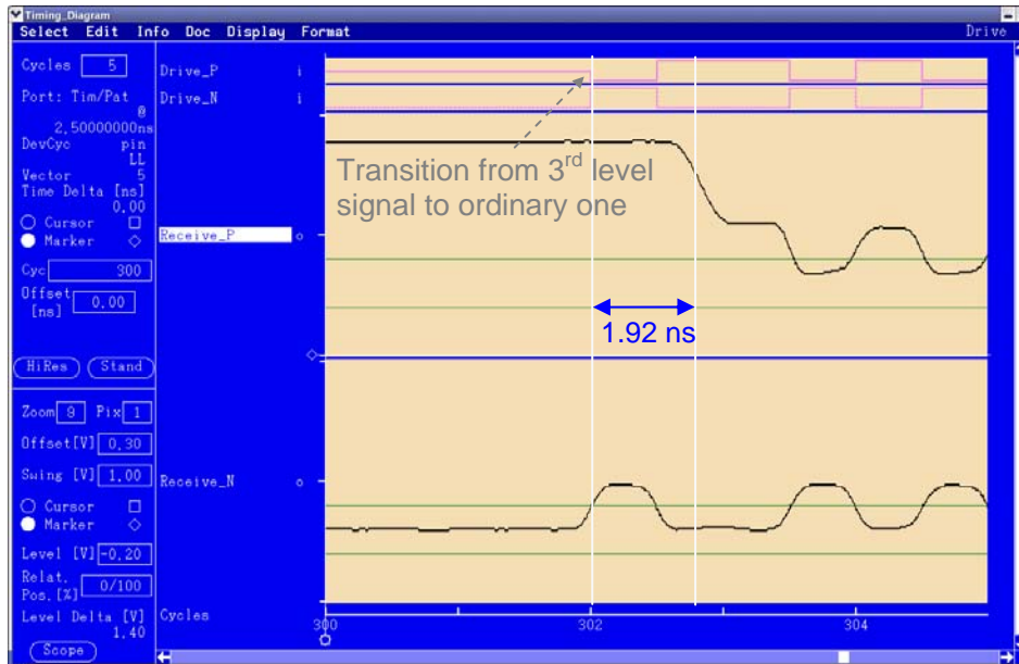
Figure 9: Intrinsic delay (1.92 ns) of third level off
