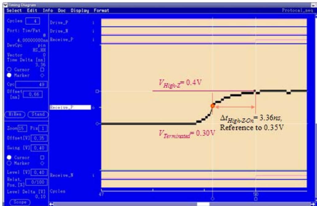
Figure 7: Switch into unterminated ATE Rx mode (uncompensated)
