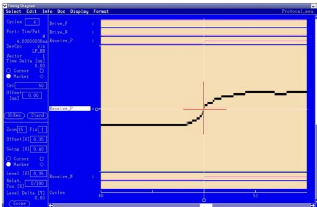
Figure 10: Switch into unterminated ATE Rx mode (compensated)
